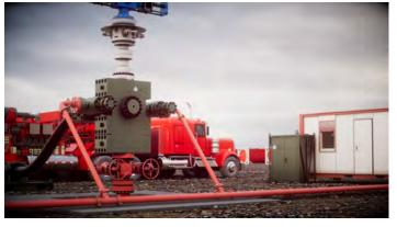
Shown above the StackLite SGV FRAC7 7-1/16" 15psi RWP tree is shown in the foreground. The compact height allows all connections to be made-up with-out working at heights.
