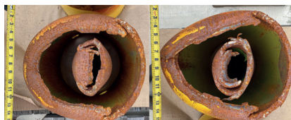
16" OD HP Casing, Q125 6-5/8" OD Inner String, V150 Combined 186ppf
